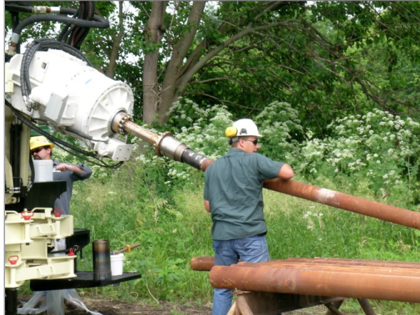
Layne's Sonic Rig was used for exploratory drilling and drilling monitoring wells.
