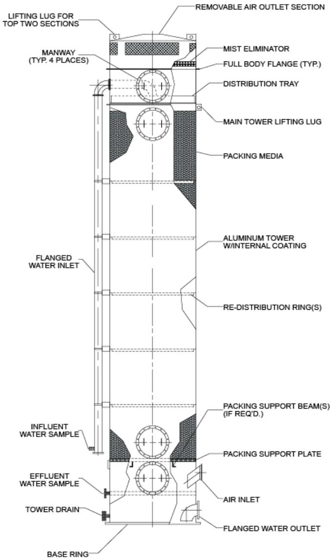
Note: Tower shown is a sample. Numerous configurations are possible for size and placement of various elements.
